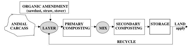
Figure 2. Material flow in dead animal composting. Forced aeration is not used. Materials are not mixed until flesh of the animal body is completely decomposed. Time can vary from 10 days (poultry) to over 100 days (> 400 lb animal).
