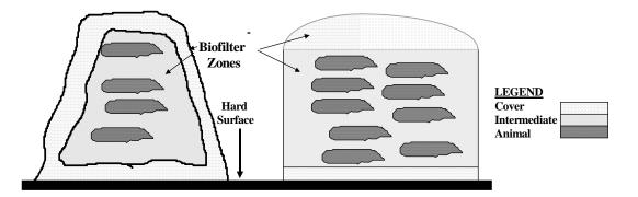
Figure 3. Cross Section Views of Composting in a Windrow or Bin for Animal Mortality. Layered animal carcasses are surrounded by material that not only provides carbon (energy) for the microorganisms, but also acts as a biofilter. Pile shape will depend on whether done in the open or in a bin.
